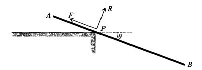
A uniform rod AB has mass m and length 2a. The point P on the rod is such that  $AP = \frac{2}{3}a$ . The rod is placed in a horizontal position perpendicular to the edge of a rough horizontal table, with AP in contact with the table and PB overhanging the edge. The rod is released from rest in this position. When it has rotated through an angle  $\theta$ , and no slipping has occurred at P, the normal reaction acting on the rod at P is R and the frictional force is P (see diagram).
