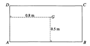
A non-uniform rectangular lamina ABCD has mass 6 kg. The centre of mass G of the lamina is 0.8 m from the side AD and 0.5 m from the side AB (see diagram). The moment of inertia of the lamina about AD is  $6.2 \, \text{kg m}^2$  and the moment of inertia of the lamina about AB is  $2.8 \, \text{kg m}^2$ .
